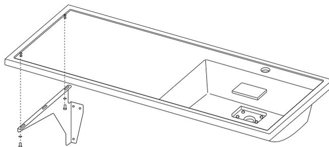
1. Pre-mark the wall on which the sink will be mounted, taking into account the layout of a sink and washing machine. Maximum washing machine depth recommended by the manufacturer, it depends on sink model; minimal distance between the washing machine and the Paola sink is 15 mm.
